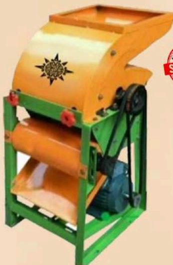
SA-CORN3 CORN PEELER CUM THRESHER [ CORN THRESHER MOTOR OPERATED ] CAPACITY - 800 KG/HR POWER -3 HP SINGLE PHASE
