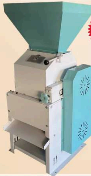
SA-CF1 CORN FLATTENING/FLAKES MACHINE POWER - 4 HP SINGLE PHASE CAPACITY - 200-250 KG/HR SUITABLE FOR - CORN/CHANA/ RICE/WHEAT/SOYA BEAN
