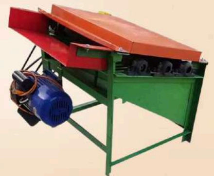
SUNFLOWER SEED THRESHER POWER- 3 HP SINGLE PHASE CAPACITY- 200 KG/HR
